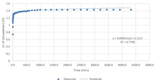
Figure 3.1 Graph log (drawdown) versus Time in minutes with predicted log regression line when Q=12.2m<sup>3</sup>/hr.
