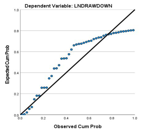
The normal probability plot of the residuals is approximately linear supporting the condition that the error terms are normally distributed when pumping rate,  $Q=51.6m^3/hr$ .
