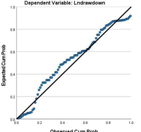
The normal probability plot of the residuals is approximately linear supporting the condition that the error terms are normally distributed when pumping rate,  $Q=12.2m^3/hr$ .
