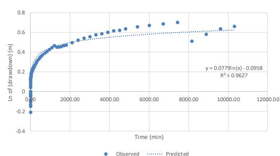
Figure 3.3 Graph log (drawdown) versus Time in minutes with predicted log regression line when Q=90.2m3/hr.
