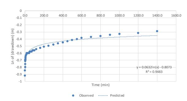
Figure 3.2 Graph log (drawdown) versus Time in minutes with predicted log regression line when Q=51.6m<sup>3</sup>/hr.
