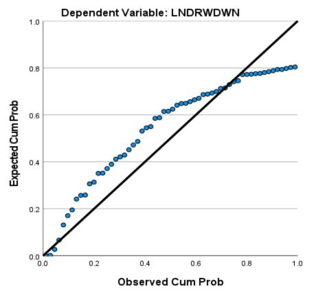
The normal probability plot of the residuals is approximately linear supporting the condition that the error terms are normally distributed when pumping rate,  $Q=90.2m^3/hr$ .
